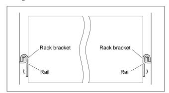
7. Fix the unit to the rack with the specified screws.
